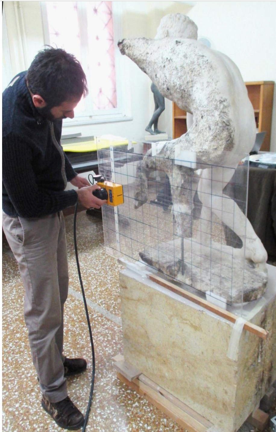
Figure 2 The process of scanning one specific area of the statue "Wrestler of Antikythera"
