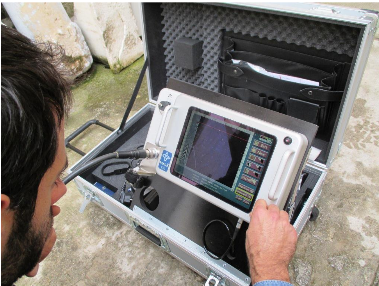
Figure 1 Calculation of the propagation velocity in the marble using the method of "hyperbola fitting" of the 3D-Vision software
