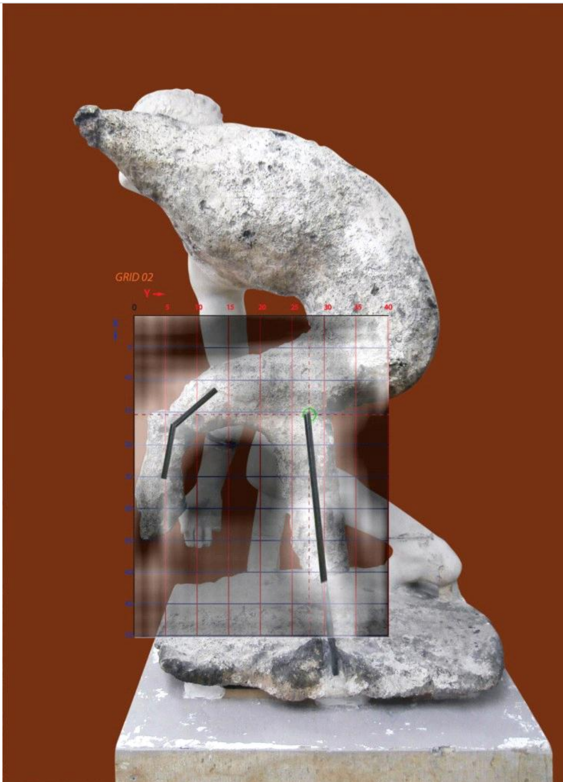
Figure 3 Superposition of the raster image from the GPR scan on the statue (Wrestler of Antikythera)
